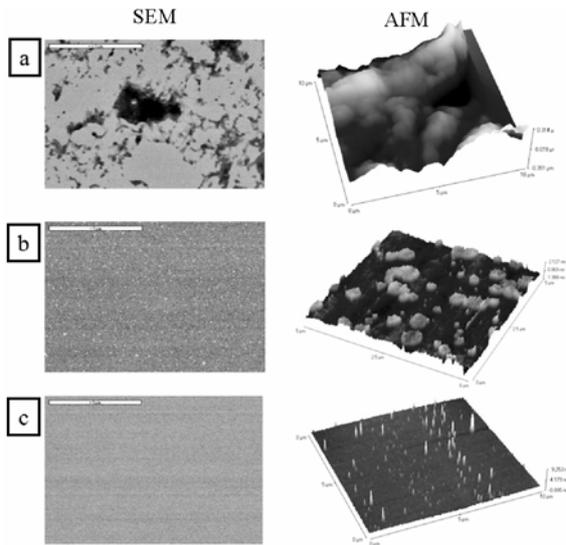
**Fig. 3.** SEM and AFM images of Si-Al thin film sputtered by Si-30wt.%Al target with different working power: (a) 1,000W; (b) 500W; and (c) 300W.
