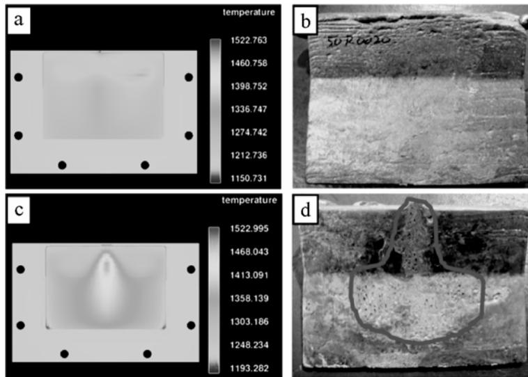
Fig. 9. Relation between the temperature distribution of melt and shrinkage pores on the surface of an ingot.
