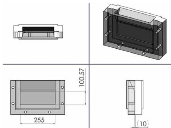
Fig. 1. Schema of casting mold plotted by Solidworks software. (unit:mm)
