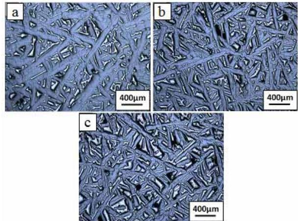
**Fig. 4.** The OM image of Si-Al targets containing different Al contents: (a) 25wt.%; (b) 30wt.%; (c) 35wt.%
