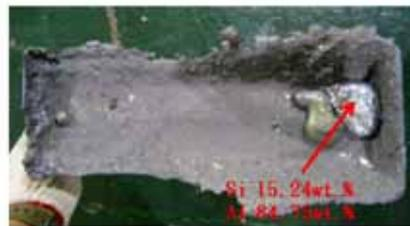
**Fig. 5.** (a) Si-Al phase diagram; (b) The macro-segregation of Si-Al ingot.
