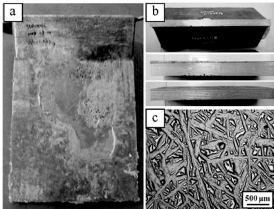
**Fig. 13.** Shrinkage pores on the (a) surface and (b) center of Si-30wt.%Al ingot cast with the condition of 1270 casting temperature and 50 mold temperature. (c) OM observation and the distribution of shrinkage pores.
