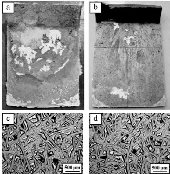
**Fig. 12.** Surface condition of the Si-30wt.%Al ingot cast with the condition of 1300 casting temperature and (a) 250 mold temperature, (b) 150 mold temperature. (c),(d) OM observation and the distribution of shrinkage pores at 250 and 150 mold temperature, respectively.
