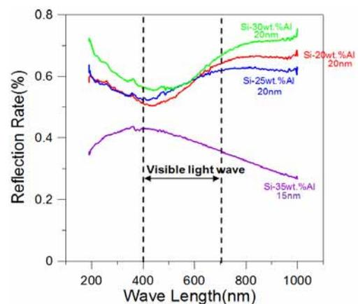
Fig. 2. Reflection rate of Si-Al thin films with different Al contents.
