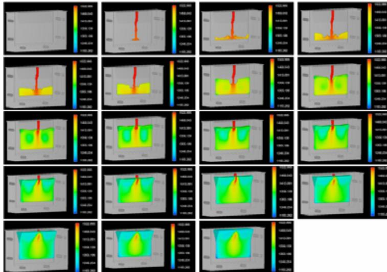
Fig. 8. Temperature distribution of melt cast onto the riser with subsequent flow into the mold cavity.
