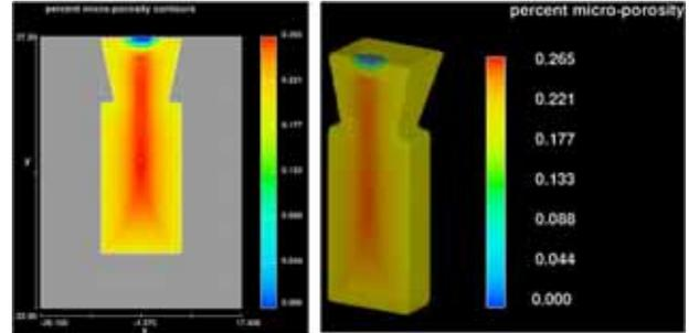
Fig. 6. Results of Flow-3D simulation of Si-Al alloy cast into a thick mold.
