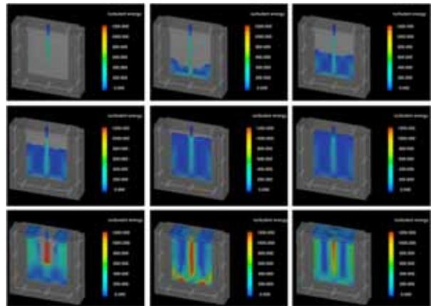
**Fig. 15.** Simulation results of the turbulent energy of suddenly increasing melt flow.
