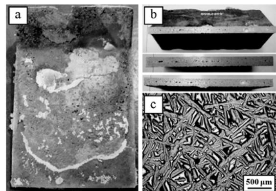
Fig. 11. Shrinkage pores on the (a) surface; and (b) center of Si-30wt.%Al ingot cast with the condition of 1330 °C casting temperature and 300 °C mold temperature. (c) OM observation and the distribution of shrinkage pores.
