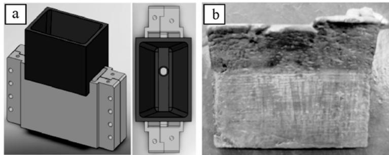
Fig. 10. (a) Schema of tundish; (b) Surface of Si-30wt.%Al ingot cast with tundish.
