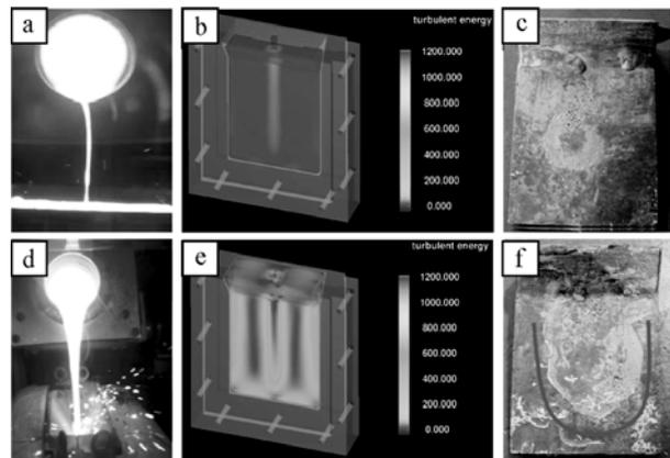
**Fig. 16.** Relation between the pouring flow of melt and the casting defect on the surface of the ingot.
