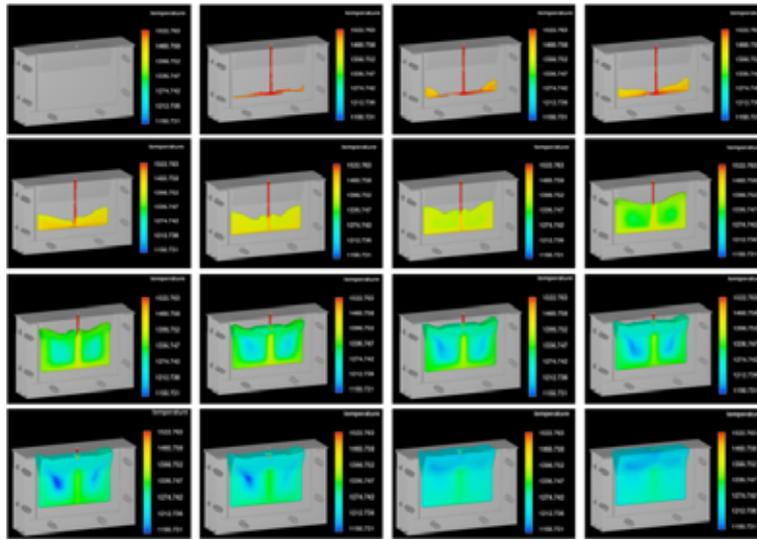
Fig. 7. Temperature distribution of melt cast into the cavity of mold directly.
